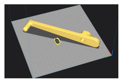
Layer Height: 0.2 (.12 looks better but optional) Wall line count: 3 Alternate extra wall: Yes Bottom Layers: 4 Top Layers: 4 Infill type: cubic Infill Density: 15% Support: No Infill Before Walls: No Build plate adhesion: skirt
