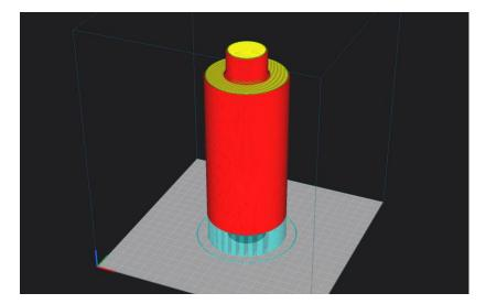
Layer Height: 0.2 Wall line count: 3 Alternate extra wall: Yes Bottom Layers: 4 Top Layers: 4 Infill type: cubic Infill Density: 15% Support: YES Infill Before Walls: No Build plate adhesion: skirt
