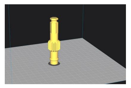
Layer Height: 0.2 Wall line count: 3 Alternate extra wall: Yes Bottom Layers: 4 Top Layers: 4 Infill type: cubic Infill Density: 100% Support: No Infill Before Walls: No Build plate adhesion: Brim
