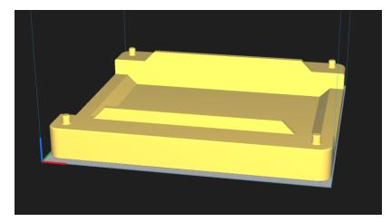
Layer Height: 0.3 Wall line count: 2 Alternate extra wall: doesn't matter Bottom Layers: 4 Top Layers: 5 Infill type: cubic Infill Density: 10% Support: No Infill Before Walls: No Build plate adhesion: skirt
