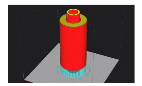
Layer Height: 0.2 Wall line count: 3 Alternate extra wall: Yes Bottom Layers: 4 Top Layers: 4 Infill type: cubic Infill Density: 15% Support: YES Infill Before Walls: No Build plate adhesion: skirt
