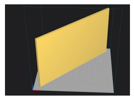
Layer Height: 0.2 Wall line count: 4 Alternate extra wall: Yes Bottom Layers: 4 Top Layers: 4 Infill type: cubic Infill Density: 25% Support: No Infill Before Walls: No Build plate adhesion: skirt
