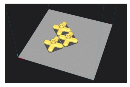
Layer Height: 0.2 Wall line count: 3 Alternate extra wall: Yes Bottom Layers: 4 Top Layers: 4 Infill type: cubic Infill Density: 15% Support: No Infill Before Walls: No Build plate adhesion: skirt
