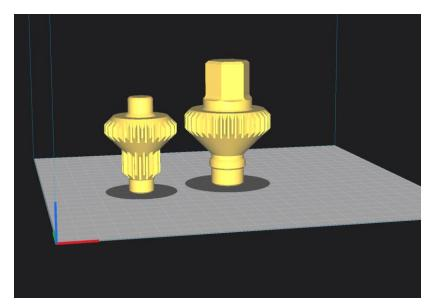
Layer Height: 0.2 Wall line count: 3 Alternate extra wall: Yes Bottom Layers: 4 Top Layers: 4 Infill type: Triangle Infill Density: 20% Support: No Infill Before Walls: No Build plate adhesion: Brim
