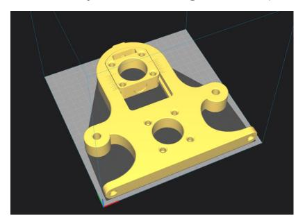
Layer Height: 0.2 Wall line count: 3 Alternate extra wall: Yes Bottom Layers: 4 Top Layers: 4 Infill type: cubic Infill Density: 25% Support: No Infill Before Walls: No Build plate adhesion: skirt
