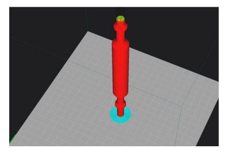
Layer Height: 0.2 Wall line count: 3 Alternate extra wall: Yes Bottom Layers: 4 Top Layers: 4 Infill type: Triangle Infill Density: 15% Support: No Infill Before Walls: No Build plate adhesion: Brim
