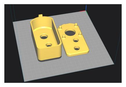
Layer Height: 0.2 Wall line count: 3 Alternate extra wall: Yes Bottom Layers: 4 Top Layers: 4 Infill type: cubic Infill Density: 15% Support: No Infill Before Walls: No Build plate adhesion: skirt
